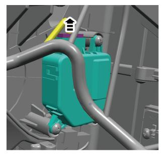
3. Remove 3 mounting screws of front passenger seat temperature air vent motor, and remove the front passenger seat temperature air vent motor.
