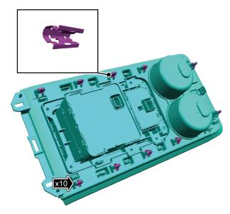
5. Disconnect the console moulding switch harness connector and remove the console moulding switch panel assembly-rear.
