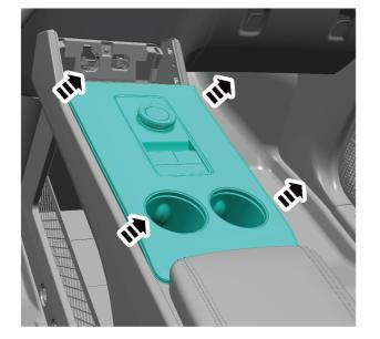
4. See the figure below for the position of the clip on the console moulding switch panel assembly-rear.
