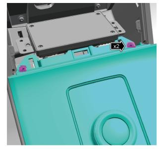
3. Remove the console moulding switch panel assembly-rear.
