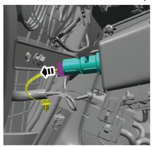
3. As shown in the figure, disconnect the mounting clip of power source socket-front, take down power source socket-front.
